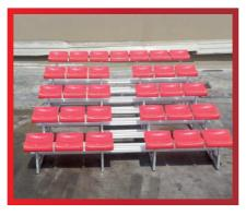
The five row bench 'Vindico II' with plastic seats and staircase is made of aluminium structure and plastic seats. The bench provides five rows of seating and has a total capacity of 31 seats. The bench measures a length of 3.1 m. The seats are made of UV protected plastic. The stairs are made from a special aluminium profile. The profiles are anodized and have an anti-slip surface. The system is dismantling and can be easily assembled at any site.
